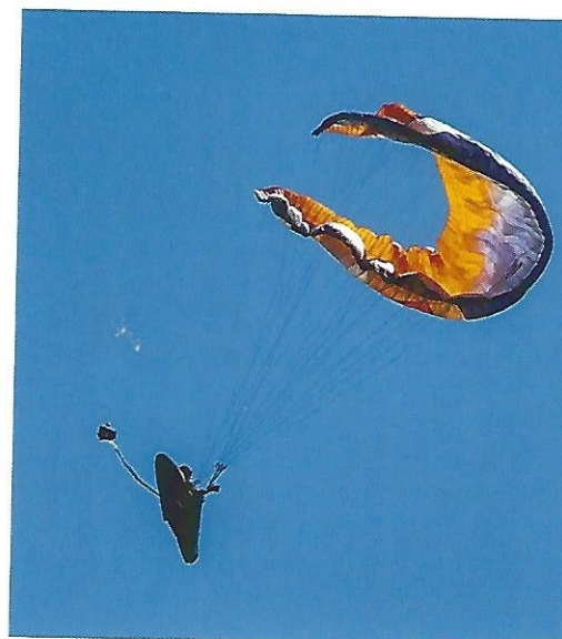
The pilot can see the glider is rotating to the right, so throws the reserve hard behind and slightly to the left. This results in the bridle being fully extended before the canopy has the chance to open
